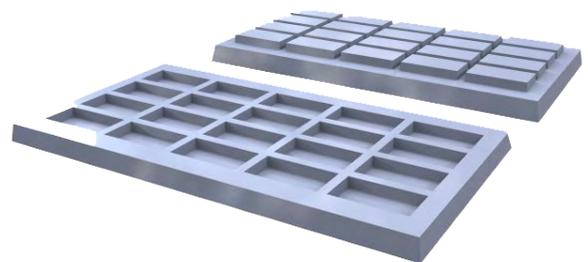
Try using a female tool instead of a male tool if webbing occurs between parts of the tool.
