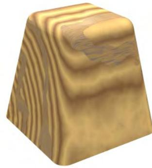
Add draught angle/radius corners to allow the material to flow over the tool/mould/pattern.
