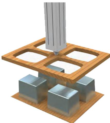
A frame attached to the plug assist that comes down as the table is raised helps to force the material down between the tools and reduce webbing.
