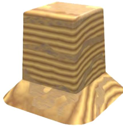
Increase tool height/add 45 degree apron to tool base to use up excess material that cause webs.
